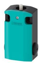
Basic switch for position switch 3SE5162 Metal enclosure XL, 56 mm wide Device connection 3x(M20 x 1.5) IP66/IP67 2 x (1 NO/2 NC) Slow-action contacts without actuator head with increased corrosion protection
