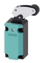
Position switch Plastic enclosure 40 mm according to EN 50041 Device connection 1 x (M20 x 1.5) 1 NO/2 NC quick action contacts Angular roller lever and plastic roller 22 mm
