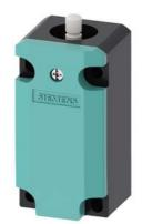
Position switch Basic switch plastic 40 mm according to EN 50041 Increased corrosion protection Device connection 1 x (M20 x 1.5) 1 NO/2 NC slow-action contacts functional at -40 °C Shock and vibration test according to EN 61373, Category 1B
