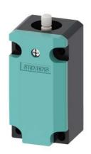
position switch basic switch plastic 40 mm according to EN 50041 increased corrosion protection device connection 1 x M20 x 1.5 1 NO/1 NC quick action contacts functional at -40  $^{\circ}\text{C}$  shock and vibration test according to DIN EN 61373, category 1B
