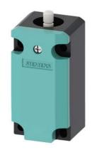
Basic switch for position switch 3SE513 Enclosure plastic according to EN 50041, 1 x (M20 x 1.5) 1 NO/1 NC quick action contacts gold-plated without actuator head
