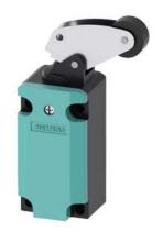
Position switch Plastic enclosure 40 mm according to EN 50041 Device connection 1x (M20 x 1.5) 1 NO/1 NC slow-action contacts Angular roller lever made of metal and plastic roller 22 mm
