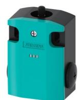
Basic switch for position switch 3SE51 Metal enclosure 56 mm wide Device connection 3x (M20x 1.5) 1 NO/2 NC quick action contacts with 2 LEDs, yellow/green 110-230 V AC without actuator head
