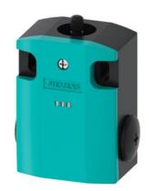
Basic switch for position switch 3SE51 Metal enclosure 56 mm wide Device connection 3x (M20x 1.5) 1 NO/2 NC slow-action contacts with 2 LEDs, yellow/green 110-230 V AC without actuator head
