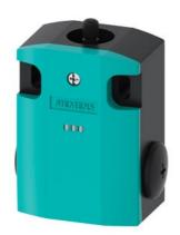
Basic switch for position switch 3SE51 Metal enclosure 56 mm wide Device connection 3 x (M20 x 1.5) 1 NO/2 NC quick action contacts with 2 LEDs, yellow/green, 24 V DC without actuator head
