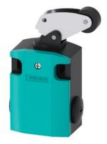
Position switch Metal enclosure 56 mm wide Device connection 3x (M20x 1.5) 2 NO/1 NC slow-action contacts Angular roller lever, metal lever and plastic roller 22 mm
