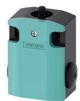
Basic switch for position switch 3SE5112 Metal enclosure 56 mm increased corrosion protection (increased corrosion protection) 3x (M20x 1.5) 1 NO/2 NC slow-action contacts with make-before-break without actuator head
