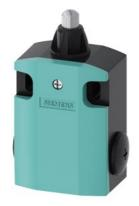
Position switch Metal enclosure 56 mm wide Device connection 3x (M20x 1.5) 1 NO/2 NC quick action contacts Rounded plunger with overtravel made of stainless steel
