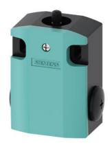
Position switch Basic switch Metal, 56 mm Increased corrosion protection Device connection 3 x (M20 x 1.5) 1 NO/2 NC slow-action contacts functional at -40  $^{\circ}\text{C}$  Shock and vibration test according to EN 61373, Category 1B
