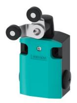
Position switch Metal enclosure 56 mm wide Device connection  $3x \, (M20x \, 1.5) \, 1$  NO/1 NC quick action contacts Fork lever operating mechanism with metal lever and plastic rollers 19 mm
