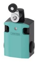
Position switch Metal enclosure 56 mm wide Device connection  $3x \, (M20x \, 1.5) \, 1$  NO/1 NC quick action contacts Rotary actuator right/left adjustable, with metal lever 27 mm long and plastic roller 19 mm
