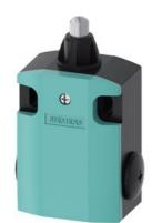
Position switch Metal enclosure 56 mm wide, Device connection 3x (M20x 1.5) 1 NO/1 NC quick action contacts, Rounded plunger, with 3 mm overtravel, made of stainless steel
