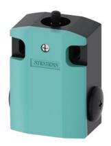
Basic switch with increased corrosion protection for position switch 3SE51 Metal enclosure 56 mm Device connection 3x (M20x 1.5) 1 NO/1 NC quick action contacts without actuator head
