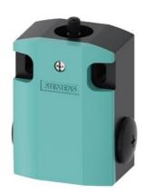
Position switch Basic switch Metal, 56 mm Increased corrosion protection 1 NO/1 NC quick action contacts functional at -40  $^{\circ}\text{C}$  Shock and vibration test according to EN 61373, Category 1B
