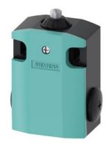
Position switch Metal enclosure 56 mm wide Device connection 3x (M20x 1.5) 1 NO/1 NC slow-action contacts Plain plunger, stainless steel
