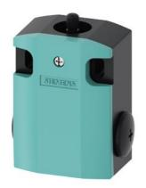
enclosure with increased corrosion protection for position switch 3SE51 56 mm wide, Metal with cover, turquoise Device connection 3 x (M20 x 1.5)
