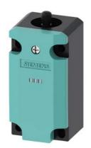
Basic switch for position switch 3SE51 Metal enclosure 40 mm according to EN 50041 Device connection 1x (M20 x 1.5) with 2 LEDs, 230 V AC yellow/green 1 NO/2 NC slow-action contacts without actuator head
