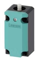
Basic switch for position switch 3SE5112 Metal enclosure, according to EN 50041 40 mm, 1 x (M20x 1.5) without actuator head 2 NO/1 NC slow-action contacts
