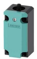
Basic switch for position switch 3SE5112 Metal enclosure 40 mm, increased corrosion protection (increased corrosion protection) according to EN 50041 Device connection 1x (M20 x 1.5) 2 NO/1 NC slow-action contacts without actuator head
