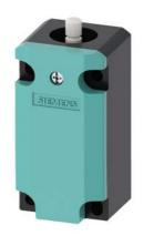
Position switch Basic switch Metal, 40 mm, according to EN 50041 Increased corrosion protection Device connection 1 x (M20 x 1.5) 1 NO/2 NC slow-action contacts functional at -40  $^{\circ}$ C Shock and vibration test according to EN 61373, Category 1B
