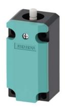
Position switch Basic switch Metal, 40 mm, according to EN 50041 Increased corrosion protection Device connection 1 x (M20 x 1.5) 1 NO/1 NC quick action contacts functional at -40  $^{\circ}$ C Shock and vibration test according to EN 61373, Category 1B
