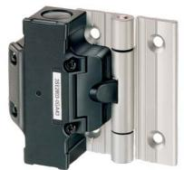
Hinge switch Molded-plastic enclosure with stainless steel hinge 2 NC/1 NO, for 40 mm profiles Supplied with additional hinge and fixing material Actuating angle  $4^\circ$
