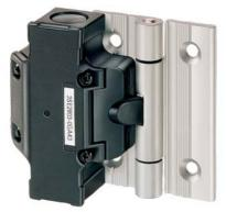
Hinge switch Molded-plastic enclosure with aluminum hinge 1 NO/2 NC, Slow-action contacts for 40 mm profiles Supplied with additional hinge and fixing material Actuating angle  $4^\circ$
