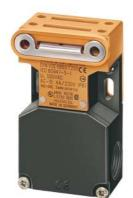
Safety position switch with separate actuator Molded-plastic enclosure, lateral and face-end operation Slow-action contacts 1 NO+2 NC, 3 x (M16 x 1.5) Pull-out force 30 N Supplied without actuator
