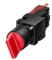
Selector switch, 16 mm, round, plastic, white, 3 switch positions I>O<II, momentary contact type, Retraction from left and right, Actuating angle 2 x 50 degree, 1 NO, 1 NO
