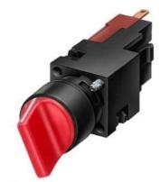
Selector switch, 16 mm, round, plastic, black, 3 switch positions I>O<II, momentary contact type, Retraction from left and right, Actuating angle 2 x 50 degree, 1 NO, 1 NO
