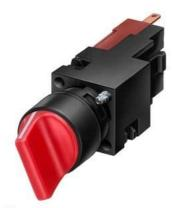
Selector switch, 16 mm, round, plastic, red, 3 switch positions I-O-II, latching, Actuating angle 2 x 62 degree, 1 NO, 1 NO  $\,$
