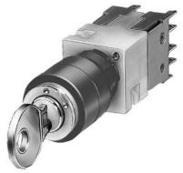
Key-operated switch, 16 mm, round, plastic, CES, 2 switch positions O-I, latching, actuating angle 62 degree, Key removal  $\rm O$
