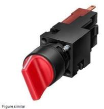
Selector switch, 16 mm, round, plastic, black, 2 switch positions O-I, latching, actuating angle 62 degree, 1 NO  $\,$
