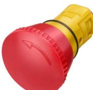
Emergency stop mushroom pushbutton, 16 mm, round, plastic, red latching, with rotate-to-unlatch mechanism, according to ISO 13850
