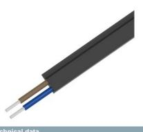
AS-i cable, shaped for external auxiliary voltage 24 V black, TPE, oil-resistant Special version according to UL Class 2, 2 x 1.5 mm2, 100 m consists of 100 m cable
