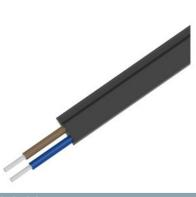
AS-i cable, shaped for external auxiliary voltage 24 V black, pure, oil-resistant 2 x 1.5 mm2, 1 km, on drum consists of 1000 m cable Shipbuilding approval
