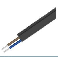
AS-i cable, shaped for external auxiliary voltage 24 V black, TPE, oil-resistant 2 x 1.5 mm2, 100 m consists of 100 m cable
