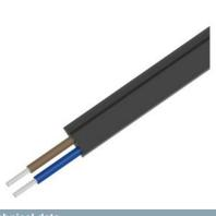
AS-i cable, shaped for external auxiliary voltage 24 V black, Rubber 2 x 1.5 mm2, 1 km, on drum consists of 1000 m cable
