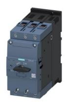
Circuit breaker size S3 for starter combination Rated current 75 A N-release 975 A screw terminal Increased switching capacity 100 kA  $\,$
