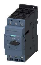
Circuit breaker size S2 for starter combination Rated current 14 A N-release 208 A screw terminal increased switching capacity
