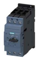
Circuit breaker size S2 for starter combination Rated current 36 A N-release 520 A screw terminal Standard switching capacity
