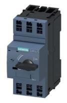
Circuit breaker size S00 for starter combination Rated current 5 A N release 65 A Spring-type terminal Standard switching capacity
