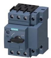
Circuit breaker size S00 for motor protection, CLASS 10 with overload relay function A-release 0.9...1.25 A N-release 16 A screw terminal Standard switching capacity
