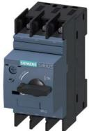
Circuit breaker size S00 for motor protection, CLASS 10 A-release 7...10 A N release 130 A ring cable lug connection Standard switching capacity
