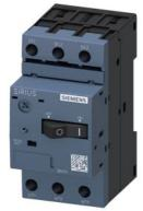
Circuit breaker size S00 for motor protection, CLASS 10 A-release 5.5...8 A N-release 104 A Screw terminal Standard switching capacity
