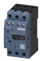
Circuit breaker size S00 for motor protection, CLASS 10 A-release 2.2...3.2 A N release 42 A 1 NO+1 NC transverse Screw terminal Standard switching capacity
