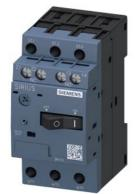
Circuit breaker size S00 for motor protection, CLASS 10 A-release 0.22...0.32 A N-release 4.2 A Screw terminal Standard switching capacity with transverse auxiliary switch 1 NO+1 NC
