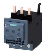
Monitoring relay, can be mounted to Contactor 3RT2, Size S2 basic, analog adjustment Apparent current monitoring 8...80 A, 50...60 Hz, 2-phase Supply 24-240 V AC/DC 1 change-over contact Monitoring for Current overshoot and undershoot Phase failure, Cable break with or without fault buffer ON delay 0-60 s Noise pulse suppression 0-30 s Switching hysteresis 6% spring-type connection system
