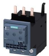
Monitoring relay, can be mounted to Contactor 3RT2, Size S2 basic, analog adjustment Apparent current monitoring 8...80 A, 50...60 Hz, 2-phase Supply 24 V AC/DC 1 change-over contact Monitoring for Current overshoot and undershoot Phase failure, Cable break with or without fault buffer ON delay 0-60 s Noise pulse suppression 0-30 s Switching hysteresis 6% spring-type connection system
