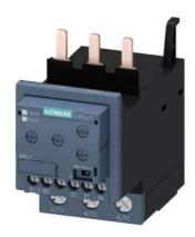
Monitoring relay, can be mounted to Contactor 3RT2, Size S2 basic, analog adjustment Apparent current monitoring 8...80 A, 50...60 Hz, 2-phase Supply 24 V AC/DC 1 change-over contact Monitoring for Current overshoot and undershoot Phase failure, Cable break with or without fault buffer ON delay 0-60 s Noise pulse suppression 0-30 s Switching hysteresis 6% Screw connection system
